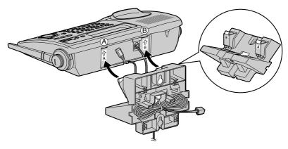
**4** Adjust the adaptor to hold the base unit, then push it in the direction of the arrow until it clicks into place.
