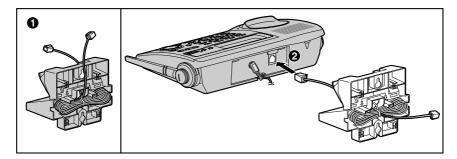
**3** Insert (A) and (B) hooks on the wall mounting adaptor into the holes on the base unit.
